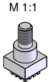
max. allowable torque for M6: 3,9Nm
