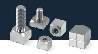
PowerOne SMD high current contacts are the result of the consequent advancement of our products for the benefit of our customers. Powerelements can be processed in the typical SMT lines and are soldered in an infrared oven or with the vapour-phase system. Depending on the layout, currents of up to 300 amperes are possible. This makes these power supply terminals ideal for use as connection elements for fuses, for cable connections to the PCB, or as fastening elements.
